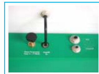
Single drop boom connections with flow control
